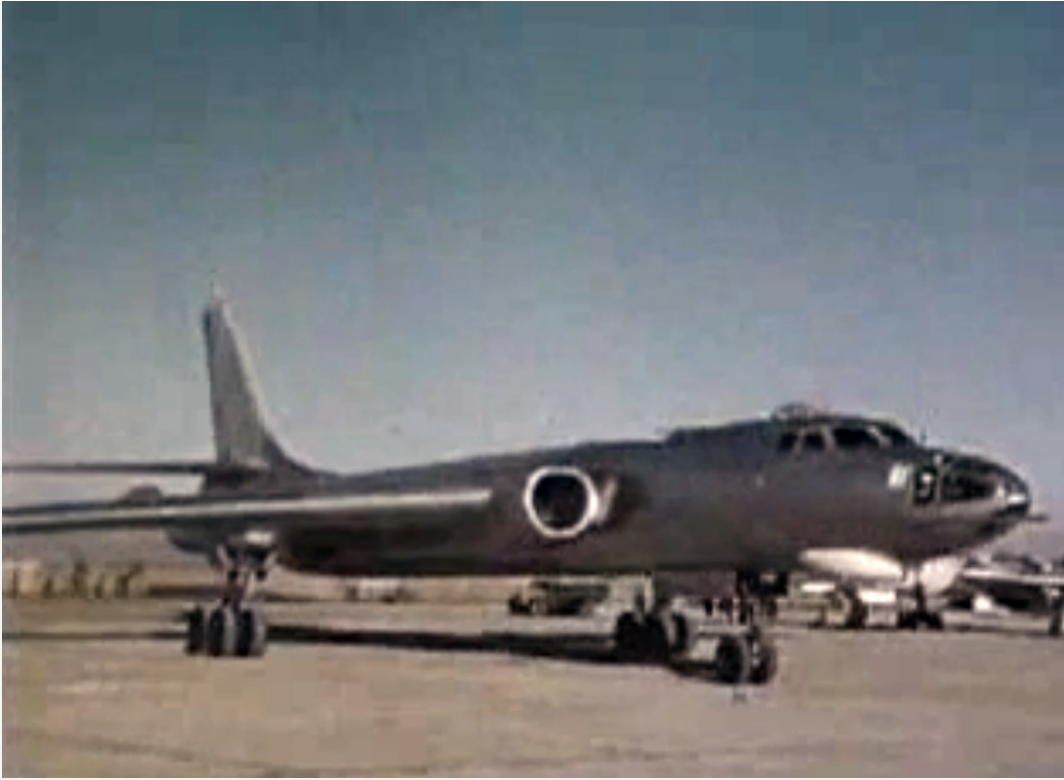
Carrier aircraft Tu-16A during tests of a bomb with an RDS-37 charge, 11/22/1955 ( source ).
